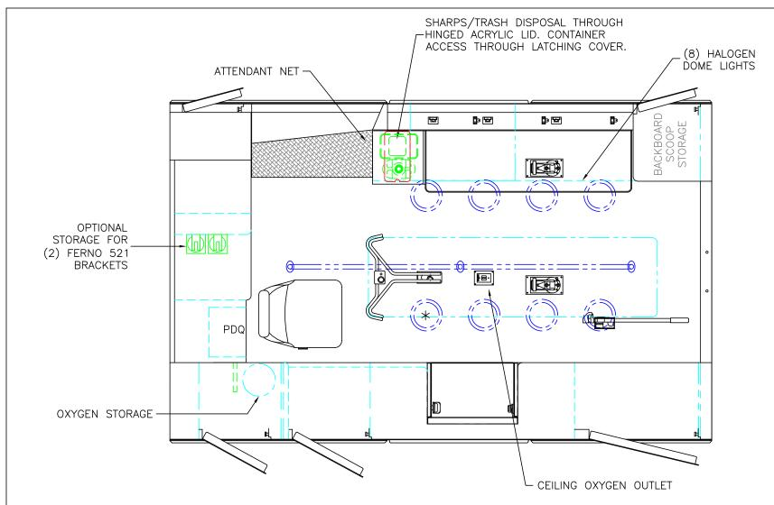
\* (1) ANTENNA BASE LOCATED OUTBOARD OF DOME LIGHT WITH COAX SERVICE LOOP
